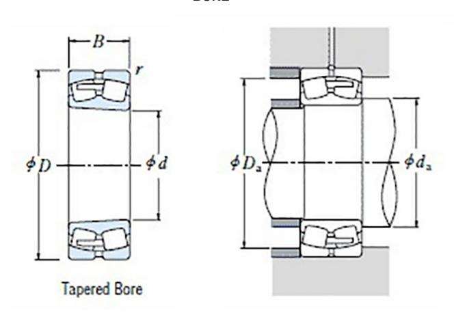
High quality spherical roller bearing with tapered bore from TIMKEN, a world leader in roller bearing technology. TIMKEN spherical roller bearings feature high class materials, innovative cage designs, enhanced surface finishes allowing better lubricant distribution and higher loadratings leading upp to lower operating temperatures and longer service life
